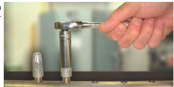
Most EXAIR Air Nozzles have a standard hex base making them easy to install with a socket wrench.
