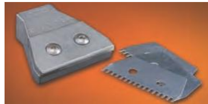
The Model 1122SS Stainless Steel Shim Set for the 2" Super Air Nozzle (shown) includes a .005" (0.13mm), .010" (0.25mm) and .020" (0.51mm) thick shim. A .015" (0.38mm) shim is installed.
