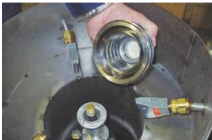
2" Super Air Nozzles blowoff metal parts as they are lifted through a vacuum chamber.
