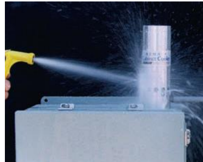
A Model 4830 NEMA 4 Cabinet Cooler cools a panel with 20°F air while keeping the inside dry.
