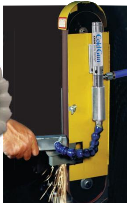
The Model 5215 Cold Gun keeps the part cool to the touch and prevents discoloration.
