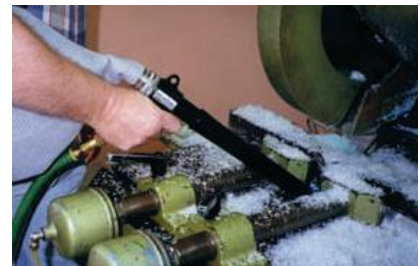
Model 6392 Vac-u-Gun All Purpose System removes plastic shavings from a saw.
