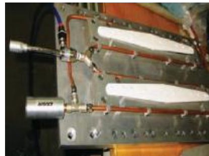
A Model 3225 Vortex Tube keeps plastic dishwasher arms cool during ultrasonic welding.
