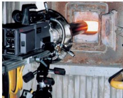
Special high temperature vortex tubes keep a boroscope lens cool while inserted into a 1200°F boiler porthole.
