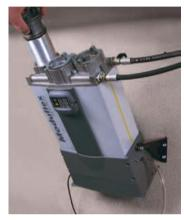
Tilt mounting kit facilitates easy cartridge replacement
