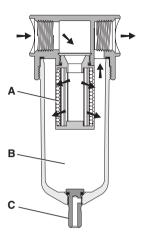
The contaminated air enters the element interior and is forced through a thick membrane (A) of "borosilicate" glass fibers coated with epoxy. Flow then passes through the element, and at this stage 99.97% of the sub micronic particles have been removed from the air stream. The tiny droplets coalesce together and are collected from the filter element by the outer drain layer.
