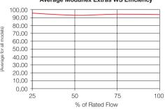
Tested with an inlet challenge concentration of 33ml/m3hr and in accordance with ISO 8573.9.
