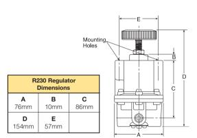
The R230 is designed for applications that require high flow capacity and accurate process control. A poppet valve which is balanced by utilizing a rolling diaphragm, insures a constant output pressure even during wide supply pressure variations. Stability of regulated pressure is maintained under varying flow conditions through the use of an aspirator tube which adjusts the air supply in accordance with the flow velocity.
