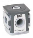
Moduflex Series Manifolds, provide up to 4 extra outlet ports, they may be assembled at any position in a combination e.g. before the lubricator to provide oil free take off or at the end of a combination to provide extra outlet ports.
