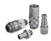
The sleeve action design requires two hand operation for added security, before the adaptor is connected. On disconnection the check unit automatically reseals the airline. When coupled the check unit allows the adaptors to swivel to eliminate kinking of the hose.
