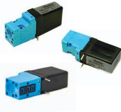
The 10mm SRS Series plastic solenoid valve converts a digital electrical signal into a digital pneumatic output. The SRS Series is constructed of engineering thermoplastics and non-corrosive metals to exceed the specifications demanded by critical applications in the life sciences.
