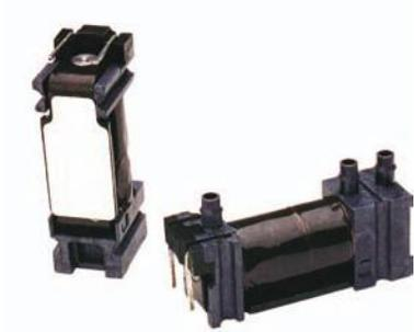
Ten-X<sup>®</sup> is a 10mm solenoid valve with a 2- or 3-way NO/NC and distributor design. Ten-X delivers repeatable “energized” and “de-energized” response times, low power, and flow capability to meet the specific performance requirements of medical devices.
