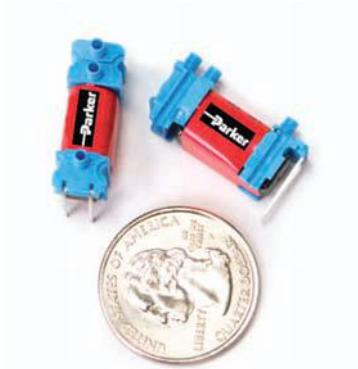
NEX-Valve is a 3 Way 2 position, bidirectional flow, non elastomeric valve that incorporates many of the proven features of the X-valve. NEX is designed to eliminate elastomer swelling commonly encountered in aggressive liquid applications.
