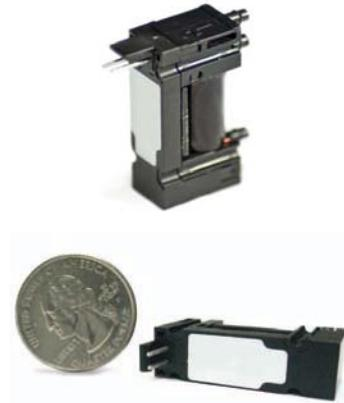
The Ten X<sup>®</sup> Le is an electro-magnetic poppet valve designed to provide the highest performance available for the package size. The quiet, lightweight 10-mm wide valve can be used stand alone with tube connections, PC or multi-station manifold mount set-ups. Integrated drive electronics featuring efficient pulse width modulation (PWM) circuit technology consume minimal power.
