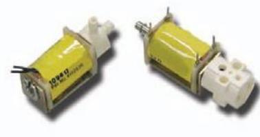
The V<sup>2</sup> valve offers a unique plastic body, which provides an economical solution without compromising on quality or reliability. Parker offers the versatile V<sup>2</sup> in either a manifold mount design or with molded barbed fittings. This PC and manifold mountable solenoid valve converts a digital electrical signal into a digital pneumatic output.
