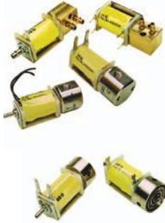
Series 11, 25, and 26 PC mountable solenoid valves convert a digital electrical signal into a digital pneumatic output. The patented miniature design is preferred by medical and analytical OEMs worldwide and allows valves to be soldered directly onto a printed circuit board, providing both electrical termination and mechanical attachment. These valves power small cylinders directly or can be used to pilot larger valves that require high flow.
