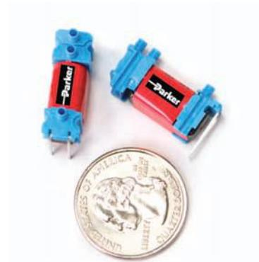
X-Valve® is a 2 or 3-way universal solenoid valve measuring just 8mm in width. The X-Valve's unitized body incorporates its functional features in a single glass-reinforced PBT (Polybutylene Terephthalate) molded body.
