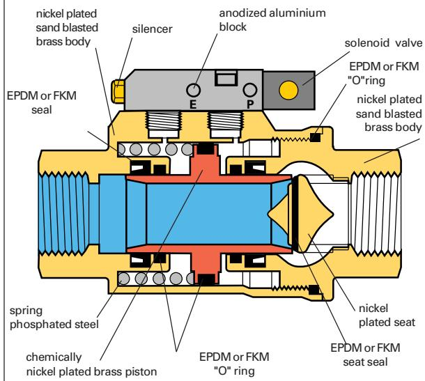
Designed with a view to overcoming the limitations of traditional actuators, the **Legris** axial valve offers the functions of a valve fitted with an actuator.
