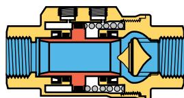
normally open axial valve in open position
