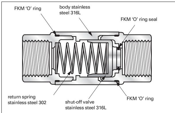
Legris stainless steel non-return valves allow air to pass in one direction whilst blocking flow in the other direction. Robust and extremely compact, they are suitable for use as a safety item in all fluids circuits. They are ideal for use in severe conditions and in aggressive environments.
