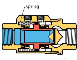
normally closed axial valve in closed position
