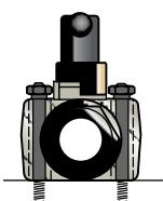
tapped fixing mounting onto a metal plate
