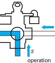
**removable handle** : where the handle is obstructed in its movement it can be refitted opposite the original position.
