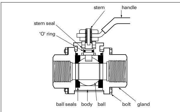
**Stainless steel series ball valves** are designed for use with corrosive fluids and in aggressive environments. Full bore, their 3-piece construction allows the valve to be disassembled in situ, to facilitate maintenance. They are suitable for higher pressure and temperature applications.
