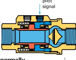
normally closed axial valve in open (actuated) position
