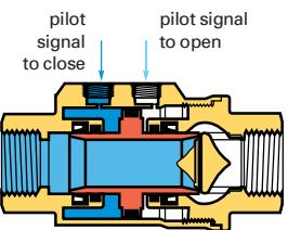
double acting axial valve in closed position
