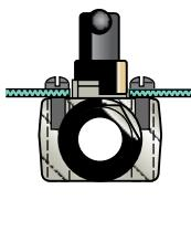
screw fixed mounting on a metal bulkhead with handle above the bulkhead
